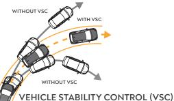
The system improves vehicle stability by detecting and reducing skidding.
