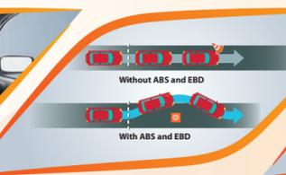
Anti-Lock Braking System and Electronic Brake Distribution
